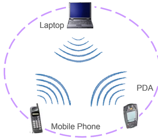
Figure 4-2. Bluetooth Ad Hoc Topology
