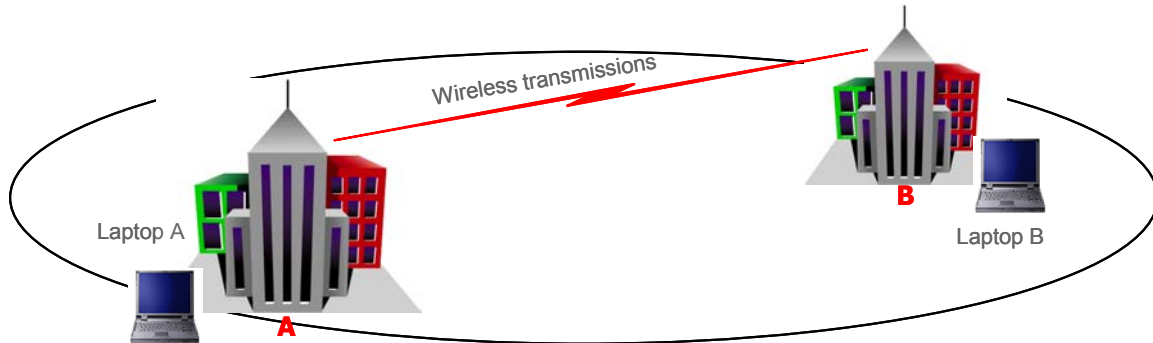
Figure 3-4. Access Point Bridging
