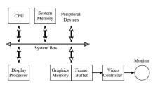
Integrated systems may be slower due to the relatively low speeds of the system bus and the greater demands placed on it, however from a programming point of view they are much neater, since all the memory can be addressed from both processors.
