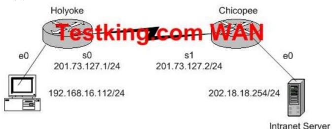
Refer to the graphic. Users on the Holyoke router are unable to access the intranet server attached to interface E0 of the Chicopee router. Inspection of the routing table of the Holyoke router shows that an entry for the Chicopee E0 network is missing.
