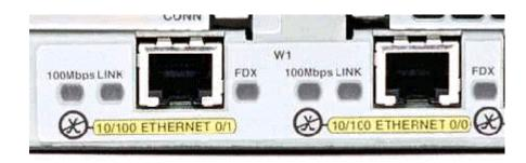
c. Identify the Ethernet ports shown that could be used for connecting the routers. Record the information below. Record the AUI port numbers if a Cisco 2500 series router is being used.
